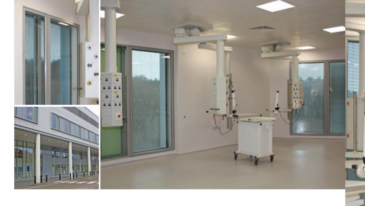
Secondary glazing with remote controlled blinds in the cavity provides privacy, additional security and helps provide a clean controlled environment to the Level 2 Neo-natal unit.
